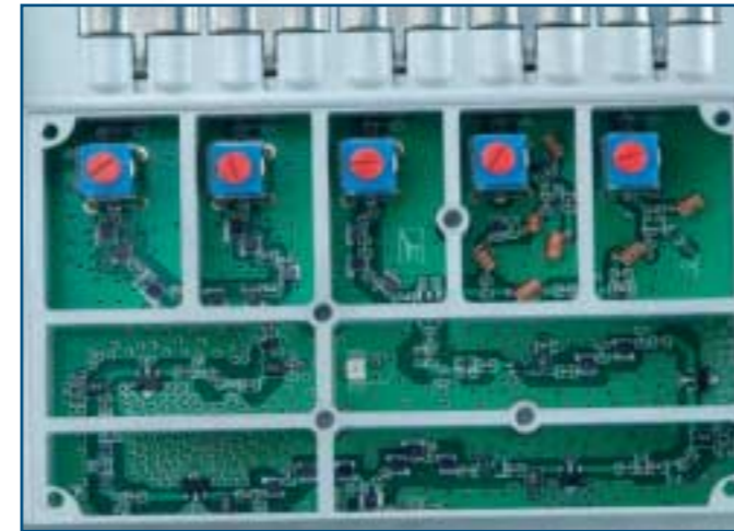
Internally, the printed circuit was separated by means of die-cast cells between each single band.
